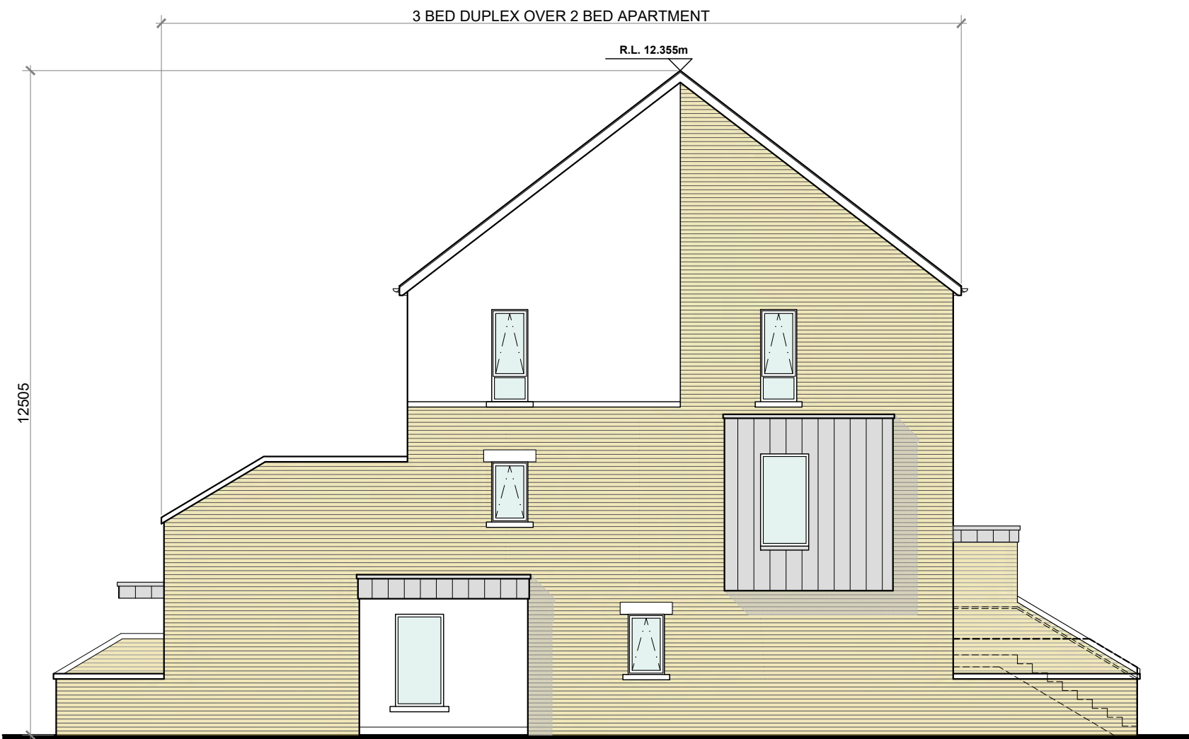
SIDE (DUAL FRONTAGE) ELEVATION @ 1:100 DUPLEX BLOCK TYPE 3B
