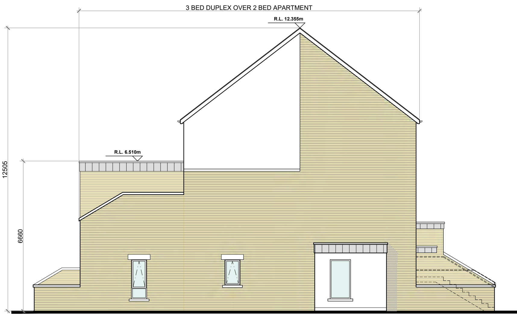
SIDE (DUAL FRONTAGE) ELEVATION @ 1:100 DUPLEX BLOCK TYPE 9
