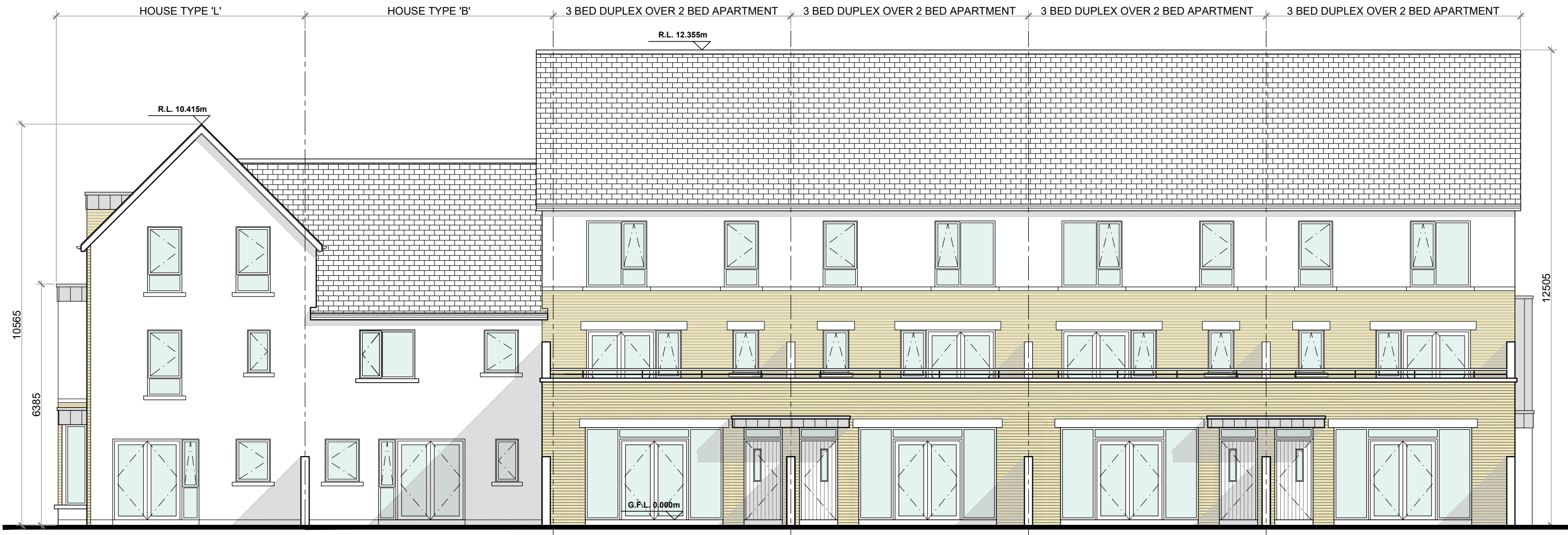
REAR ELEVATION @ 1:100 DUPLEX BLOCK TYPE 3B
